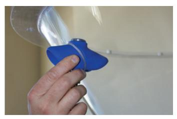
4. Fold & Insert the Fluidizer Disk into the installation hole.
