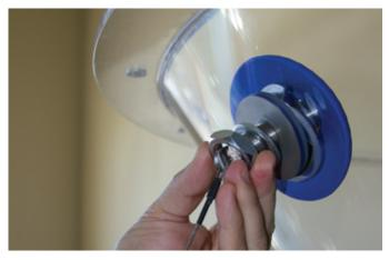
**6.** While continuing to hold retaining cable, slide the Fast-Fit™ sealing washer and the Fluidizer washer over the retaining cable and onto the stem. Next slide the nut over the retaining cable and thread it onto the stem.
